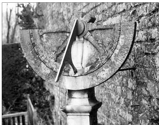
The Penshurst dial: note that most of the hour lines are visible and the metal stay to the wall. Photo: David Brown.
