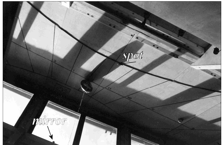
Fig. 2. View of the ceiling with the balloon strategically placed to cast a shadow for the reflected spot.
