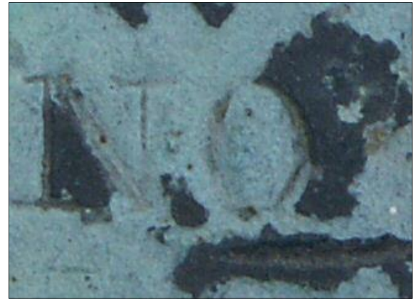
Fig. 8. Close-up of the patina and corrosion products around the 'NO' of 'ANNO', seen at approximately 4× lifesize. Notice how the black corrosion clings to the edge of the engraving.
